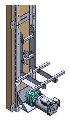
Once the assembly of the first section of track is complete, set it inside the shaft, and loosely anchor it to the wall. It is not recommended to fully secure it to the wall at this time.
